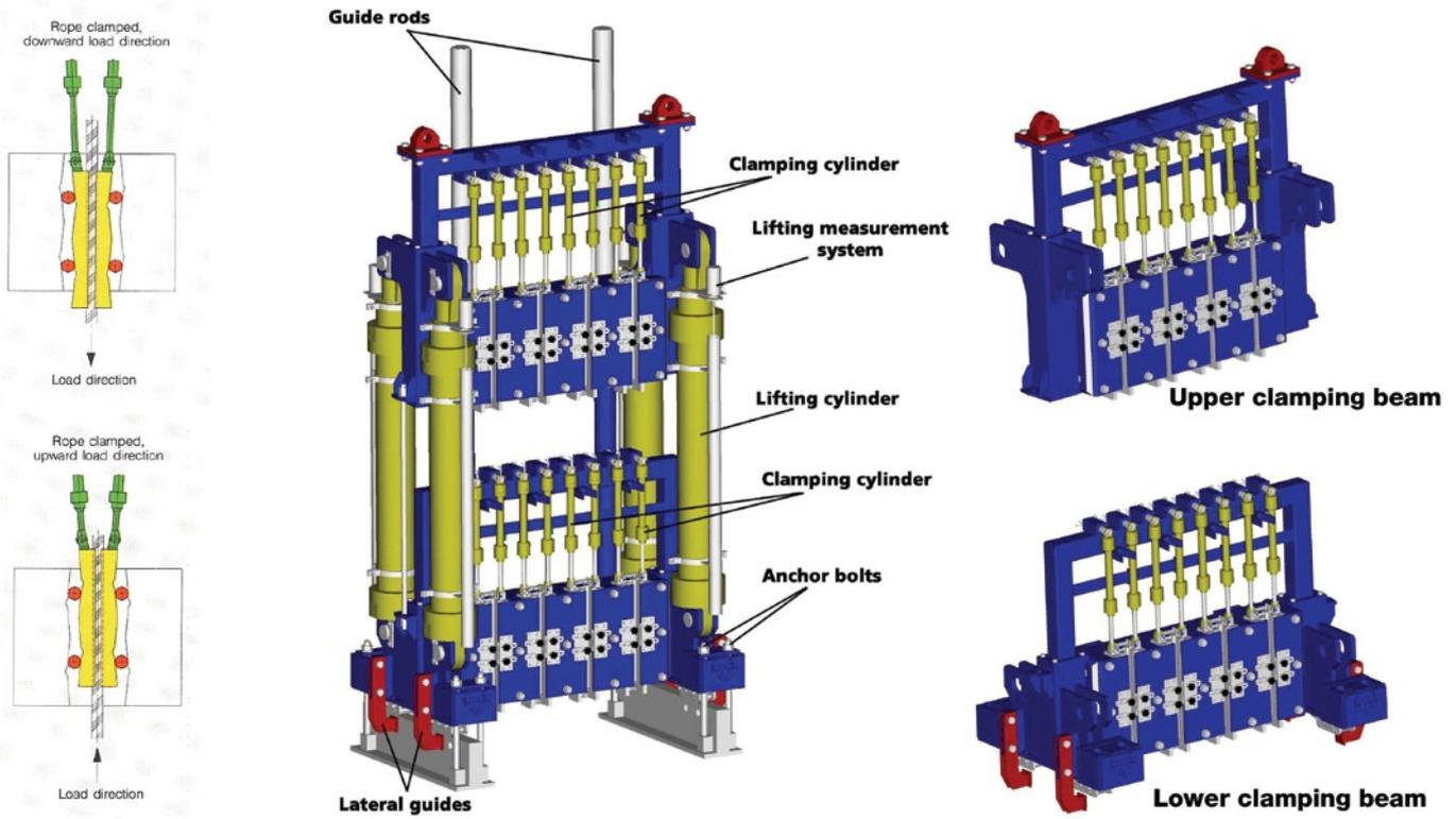
Principle of the Clamping and Lifting Device with Two-Directional Clamps
