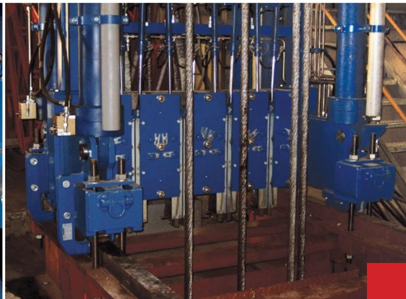
Lower Clamping Beam with Travelling Device
